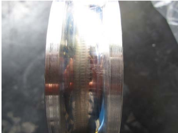
Picture 1: Inner ring tread with axial current marks (corrugation)
